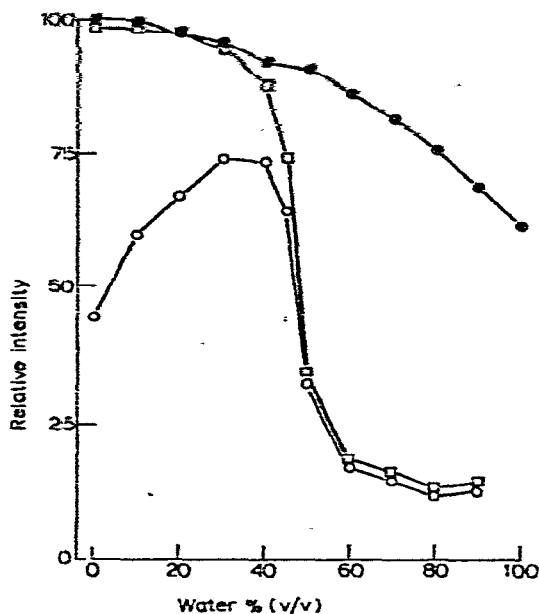
Fig. 2. Variation in fluorescence intensity, excited at 255 nm and monitored at 385 nm, with water content of aqueous methanol solutions, of the formic derivative (deoxygenated, filled circles) and the stearic derivative (deoxygenated, squares; aerated, open circles). The concentration of the derivatives was 1 \mu\text{M} .
